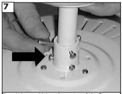
Insert downrod into yoke on top of the Fan Body. Align the hole in the Downrod with the hole in the Yoke. Insert the Pin through the Yoke and Downrod until the point appears on the other side.
